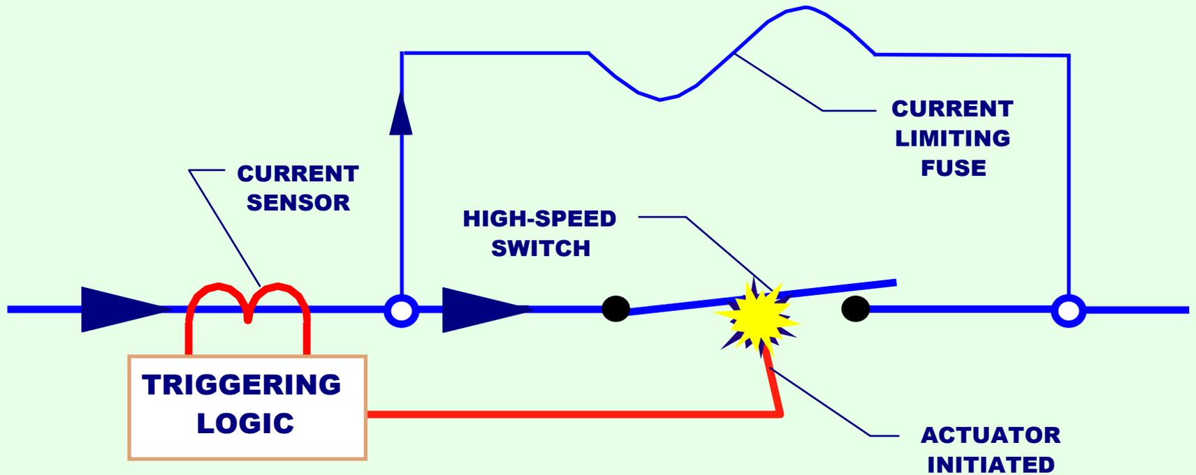
**4. SWITCH OPENING – SHUNT FUSE IS COMMUTATED INTO CIRCUIT**
