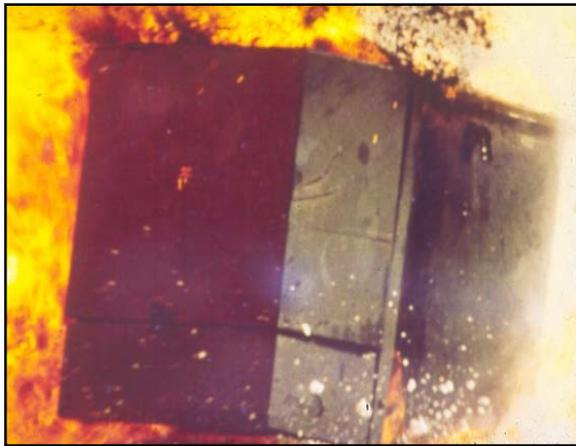
well before a circuit breaker or recloser can clear the circuit. Equipment not containing oil may still explode and evolve huge volumes of smoke and toxic gases. This may be spread through the ventilation systems of a major office complex.
